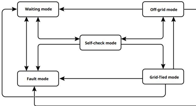
Fig. 3.6.1 Operating status of inverter
