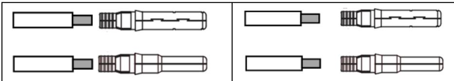
2. Loosen the terminal cover and pass the cable through the terminal cover. Insert the mold into the wiring slot until sound is given to indicate the connection in place. Tighten the terminal cover (as shown in the following figure).
