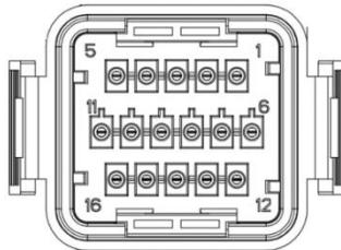
Fig. 6.5.4.1 COM communication interface
