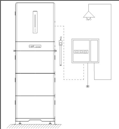
Measure the distance between the distribution box or load and the inverter by the measuring tape and select the ground cable with appropriate length.
