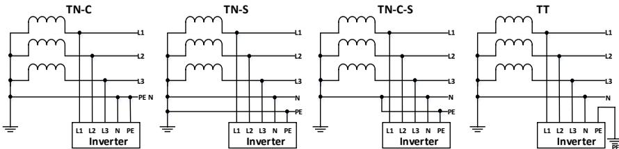
Fig. 3.4.1 Supported grid types
