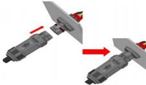
Connect the equipment with the cable while you can hear the ticking.
