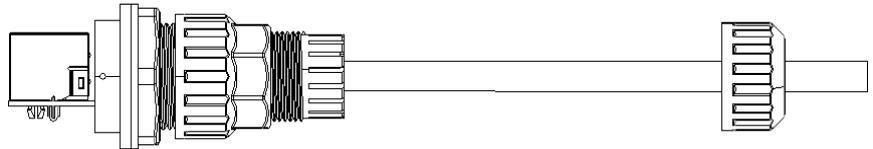
Clockwise screw the the connecting nut onto the RJ45 connector with recommended torque 2N·m;
