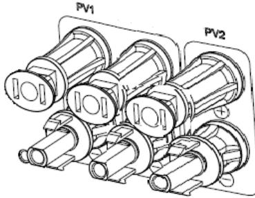
Polarity of input terminal of external input cable
