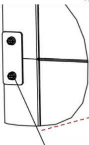
Stainless steel M4 combination screw tightened
