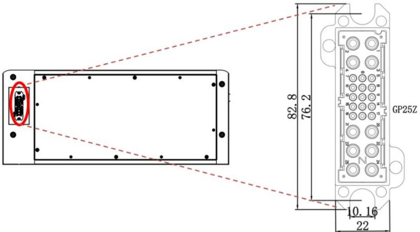
Fig. 3.7.2.3 Bottom ports of PDU-GU-Y
