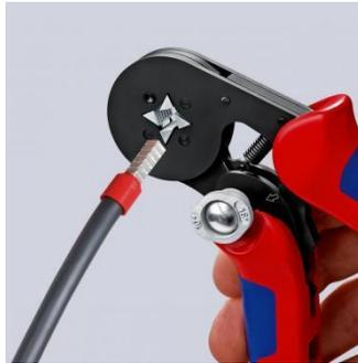
Use the terminal crimping pliers to press the pre-insulated end of the tube to the cable.
