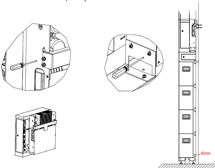
Install the hanging plate onto the power supply by M6X20 screws, stack the power supply on the distribution box by aligning with the hanging plate, connect the power supply with the distribution box by the angle iron, and fix the angle iron by M4X10 screws to complete the stacking of the battery.
