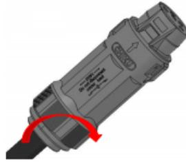
Push the clamping claw into the securing ring and screw the cable fixing nut into the housing through the torque of  $4.0 \pm 0.5 \text{ N}\cdot\text{m}$ .
