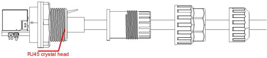
Insert the registered jack into the RJ45 connector until you hear a very clear "click";
