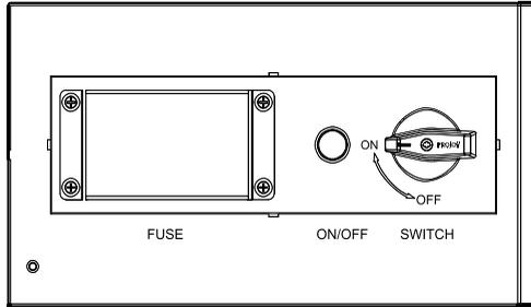
Fig. 3.7.2.4 Description of left side panel for PDU-GU-Y
