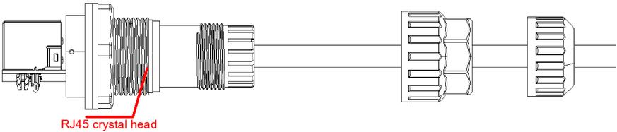
Press the fastener slightly to insert the registered jack into the RJ45 connector and contact the RJ45 connector.
