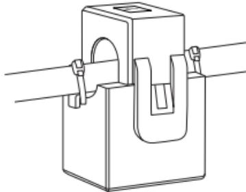
Pass the current wire through the current transformer and fix it with a cable tie.
