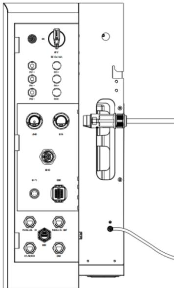
Insert the terminal into the load interface, rotate the terminal head to securely connect with the equipment, and check the connection.
