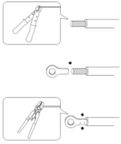
Strip 4mm insulation layer of the ground cable by the wire stripper, install the ground cable terminal, and press the ground cable terminal with the crimping pliers.
