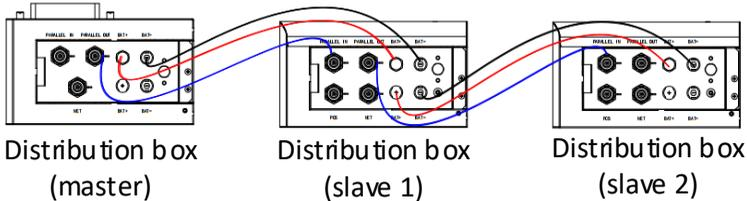
**Note:** When multiple battery packs are stacked, respectively connect 120Ω terminal resistance with the port PARALLEL IN of the first distribution box and the port PARALLEL OUT of the latest distribution box.
