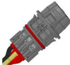
Crimp the cables, and tighten the screws at torque  $0.8 \pm 0.1 \text{ N}\cdot\text{m}$
