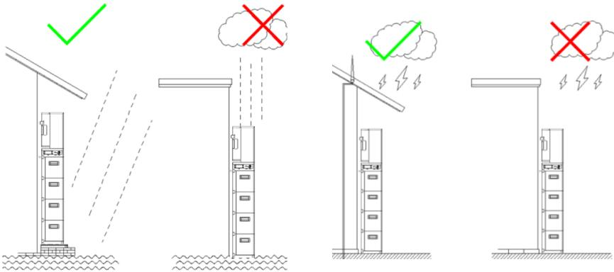
Do not install the inverter in a location which may be exposed to moisture, floor and lightning stroke.
