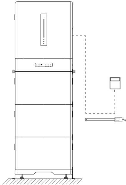
Measure the distance between the equipment and the kilowatt-hour meter by the measuring tape and select the network cable with appropriate length.
