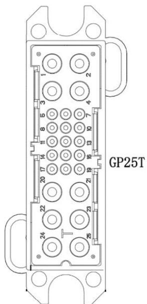
Fig. 3.7.4.2 Top ports of abutment
