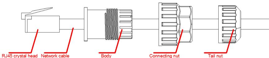
Insert the network cable into the connector components according to the figure;
