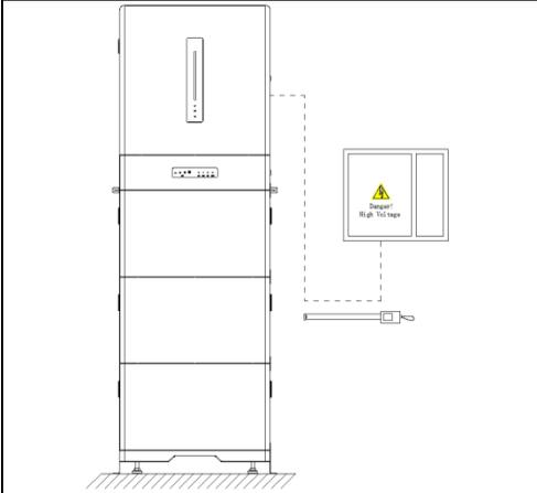
Measure the distance between the equipment and the distribution box by the measuring tape and select the ground cable with appropriate length.
