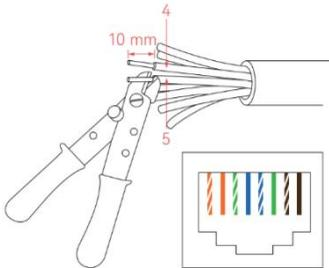
Strip 10mm insulation layer from one end of the network cables 7# (brown and white) and 8# (brown)
