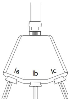
Insert the CT terminal into the adapter ports 1-3, the phase A CT plug into the 1a port, the phase B CT plug into the 1b port, and the phase C CT plug into the 1c port.
