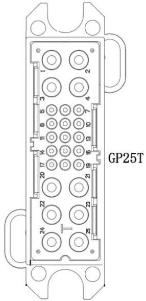
Fig. 3.7.2.2 Top ports of PDU-GU-Y
