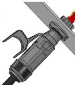
Remove the cable end from the equipment.
