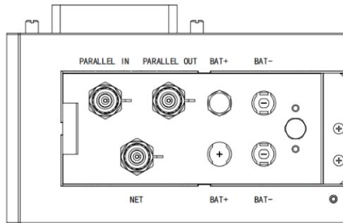
Fig. 3.7.2.5 Description of right side panel for PDU-GU-Y
