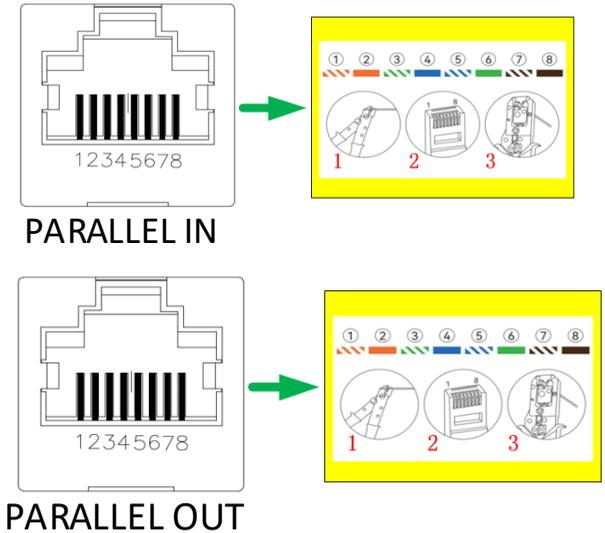
Fig. 6.5.3.1 Schematic diagram of LAN interface connection
