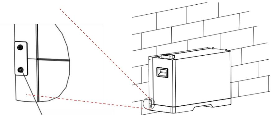
Stainless steel M4 combination screw tightened
