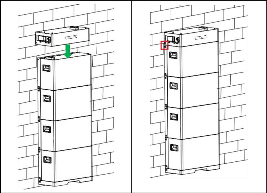
**Note: the same method is used to install the integrated and split distribution boxes**
