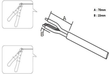
Strip 70mm cable sheath and 15mm insulation layer of the cable by the wire stripper.
