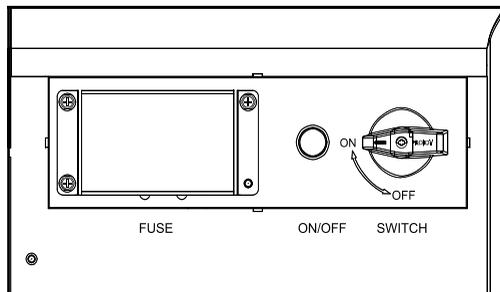
Fig. 3.7.2.9 Description of left side panel for PDU-GU-F
