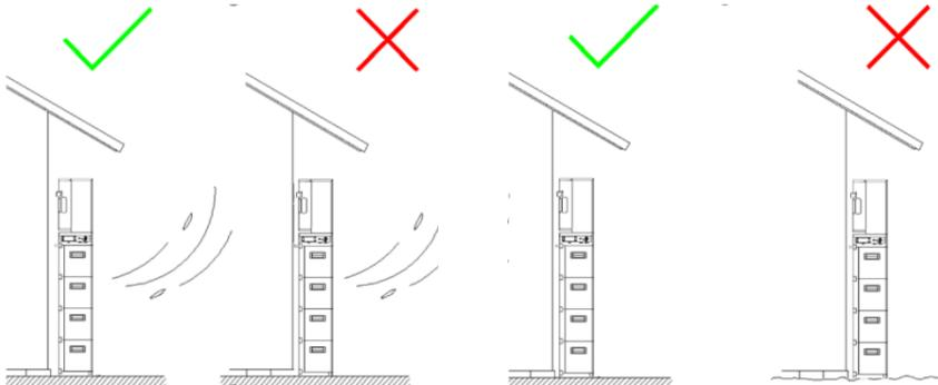
Self-cooling heat dissipation mode is used for the inverter. In order to ensure a good heat dissipation effect, install the inverter in well-ventilated environment.
