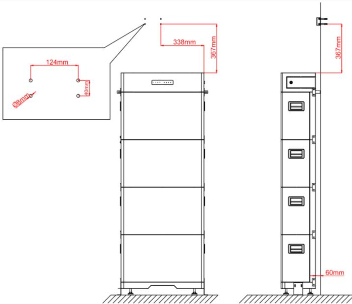
Drill the holes (about 50mm deep) on the wall with the impact drill according to the location dimensions shown in the drawing. Hammer the expansion bolt and the bushing into the bottom hole and install the wall-mounted plate by the nuts and the flat washers.
