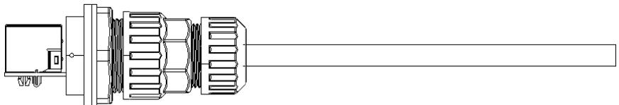
Clockwise screw the tail nut on the body with recommended torque 2N·m, and observe the wire inlet to check obvious dint on the seal ring .
