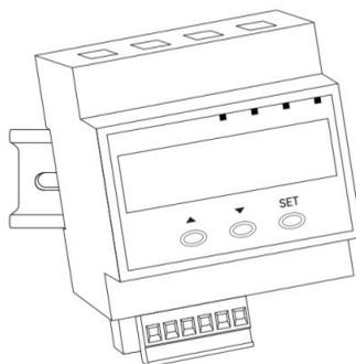
Install the kilowatt-hour meter on the guide rail.
