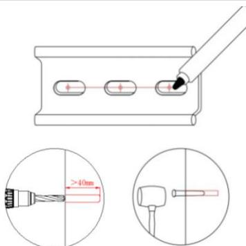
Select and mark an installation location for the kilowatt-hour meter according to the screw holes on the kilowatt-hour meter sliding rail.
