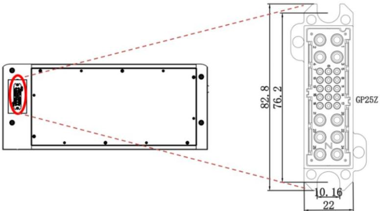
Fig. 3.7.2.7 Bottom ports of PDU-GU- F
