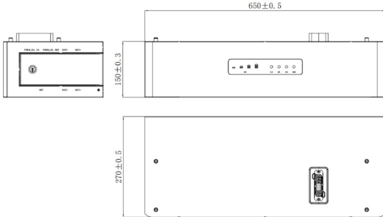
Fig. 3.7.2.1 Appearance of PDU-GU-Y
