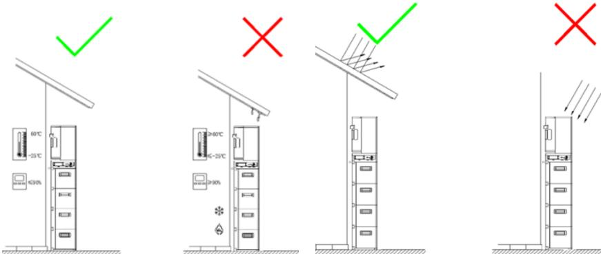
Install the inverter at  $-25$  to  $+60^{\circ}\text{C}$  and 0%-90% relative humidity (no condensation). The inverter may be installed outside away from direct sunlight.
