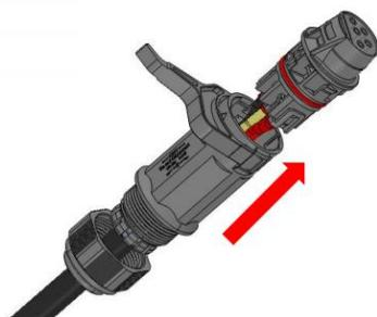
Press the unlocking position with a removal tool, pull the cable and in the arrow direction to complete the removal.
