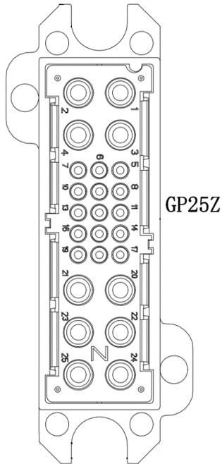
Fig. 3.7.1.1 Bottom battery ports of inverter GP25Z
