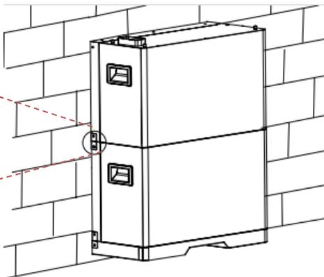
**Step 3: stack the cell and install case connecting part**
