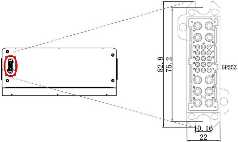
Fig. 3.7.3.3 Bottom ports for EHBS-P5-TH
