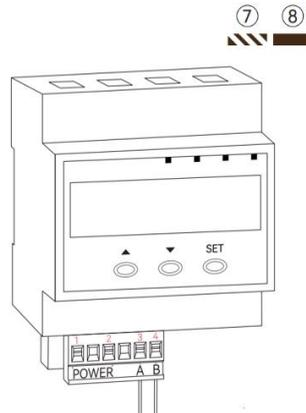
Insert the network cable 7# (brown and white) into the third port of the kilowatt-hour meter, and the network cable 8# (brown) into the fourth port of the kilowatt-hour meter, tighten the screws, and check whether the cables are connected securely .
